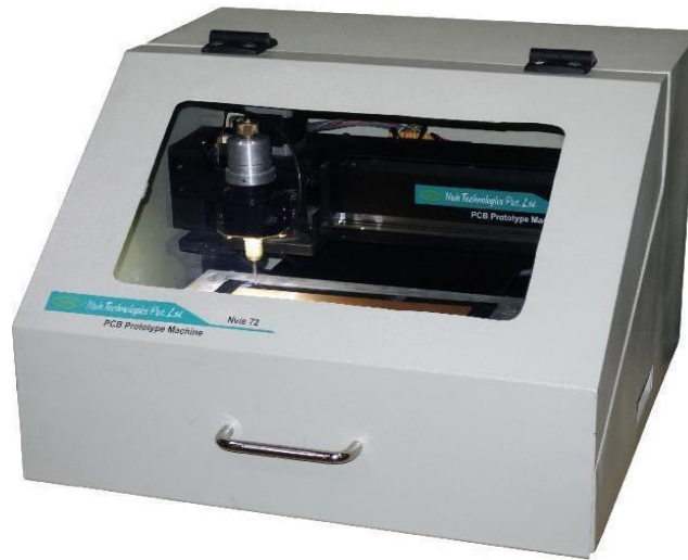
Fig 3. PCB prototype machine
